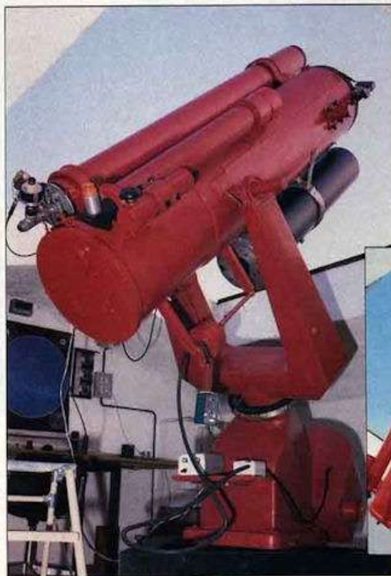
The main telescope at Luciano Lai's Giordano Bruno Observatory is this fork-mounted 0.4-meter (16-inch) f/5 Newtonian reflector. The four piggy-back instruments are 60-mm and 120-mm finders, a 150-mm f/15 guiding refractor, and the Schmidt camera (black tube) described in the text. All photographs are by the author.
